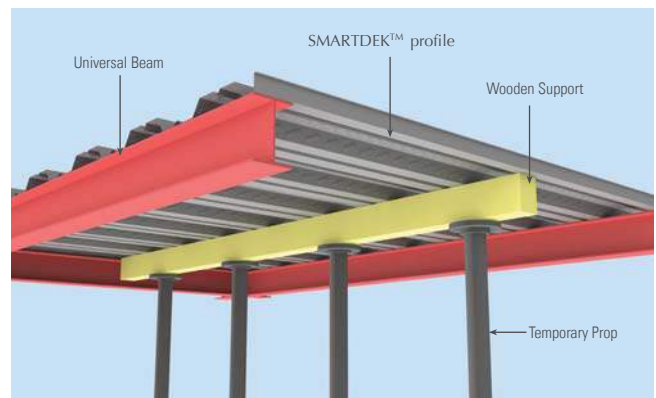
Temporary support details (If required): SMARTDEK™ profile spans longer than conventional system where possibility of temporary support is less.
