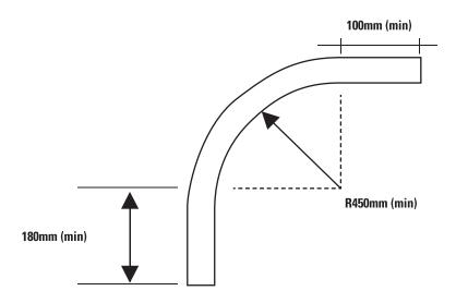
• Maximum length of sheet that can be crimp curved for ridge application is aproximately 12000mm. The curve can either be convex or concave.
