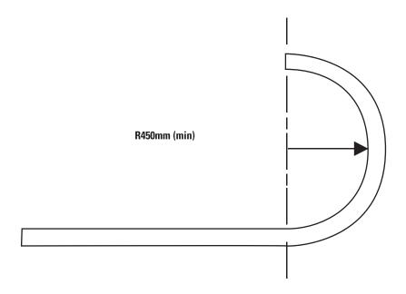
• When both ends are crimp curved, the maximum recommended straight distance between the two curves should be 6000mm.
