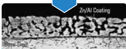
Microscopic view of TRUECORE® steel
