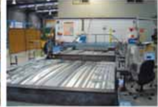
Formwork - Air Pressure Test
