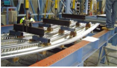
Formwork – Point Load
